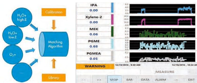
Figure 2: Schematic of the AME software data flow (left) and the user interface displaying the calculated concentrations.
