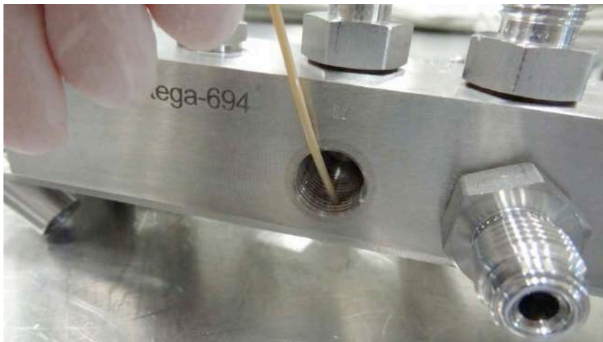
Figure 1: Contamination Analysis of Gas Manifold of an Optical Lithography Tool.
